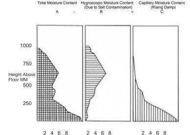
**Figure (2):** Graph (b) shows that the amount of water absorbed by the masonry from air is about 5% at 600mm above floor level. The hygroscopicity of uncontaminated masonry is 0.1-0.2%. The additional water absorption is due to salt contamination.
